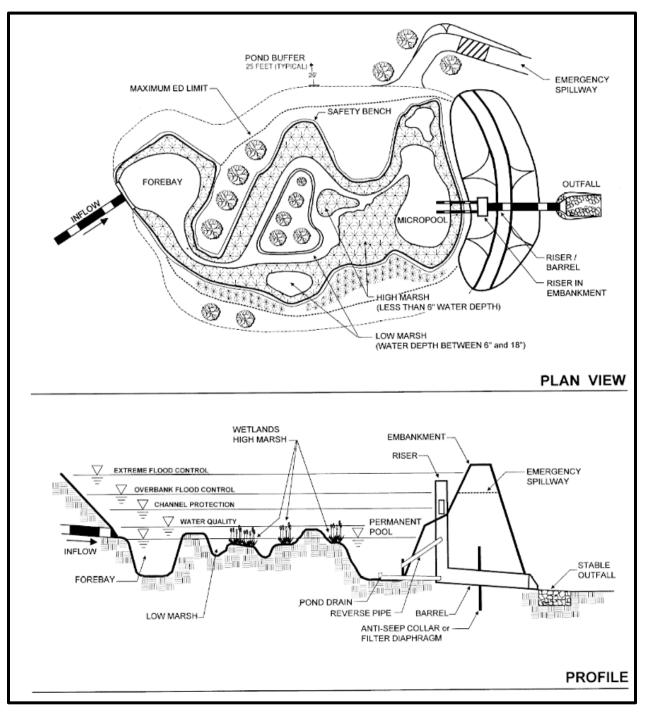
Figure 3-5. Schematic of a Typical Shallow Constructed Wetland
