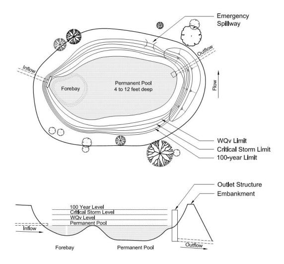
Figure 3-4. Schematic of a Wet Extended Detention Basin
