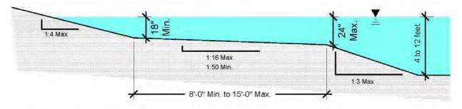
Figure 3-2. Schematic of a Submerged Bench
