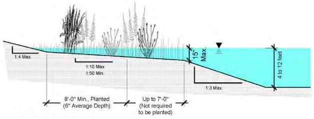
Figure 3-3. Schematic of a Submerged Bench with Plantings
