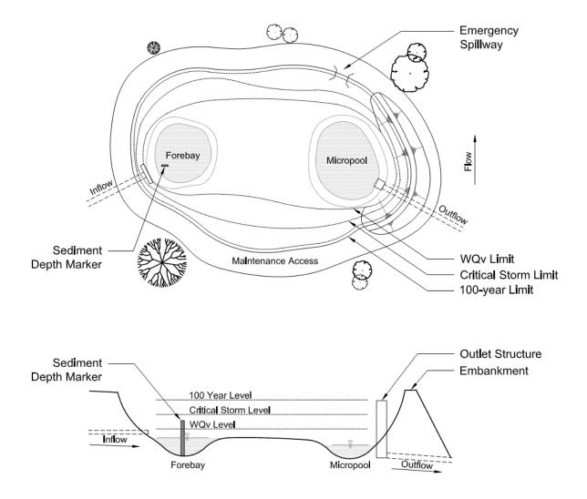
Figure 3-1. Schematic of a Dry Extended Detention Basin
